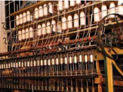
Throstle frame, c. 1835. The Lowell Machine Shop made this and many other first-generation American mill machines.
