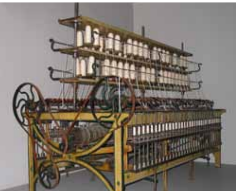
Throstle frame, c. 1835. The Lowell Machine Shop made this and many other first-generation American mill machines.
